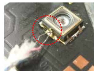
Fig. 1 Using higher heat-conductive grease or adhesive when Tj measured with thermocouples
