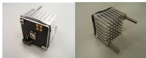
Fig. 2 Aluminum board + Heat sink
