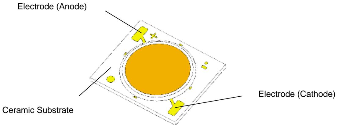
Figure 1. COB LED Structure (e.g. NFCxL060B)
