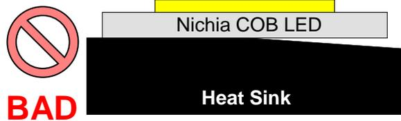
Figure 14. Insufficient Flatness for the Heat Sink Contact Surface
