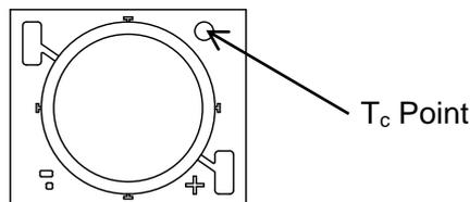
Figure 10.  $T_c$  measurement point
