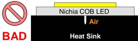
Figure 16. Heat Sinks with Screw Holes on the Contact Surface
