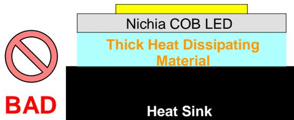
Figure 20. Excessively Thick Heat Dissipating Materials between the LEDs and Heat Sink
