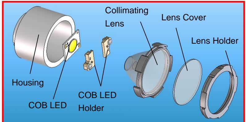
Structure of COB LED Module (Light Engine)
