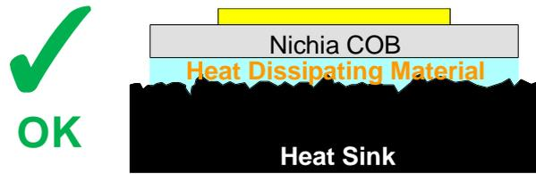
Figure 12. Heat Sinks with Uneven Contact Surfaces and Sufficient Heat Dissipating Material
