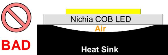
Figure 19. Heat Sinks with Curved Surfaces
