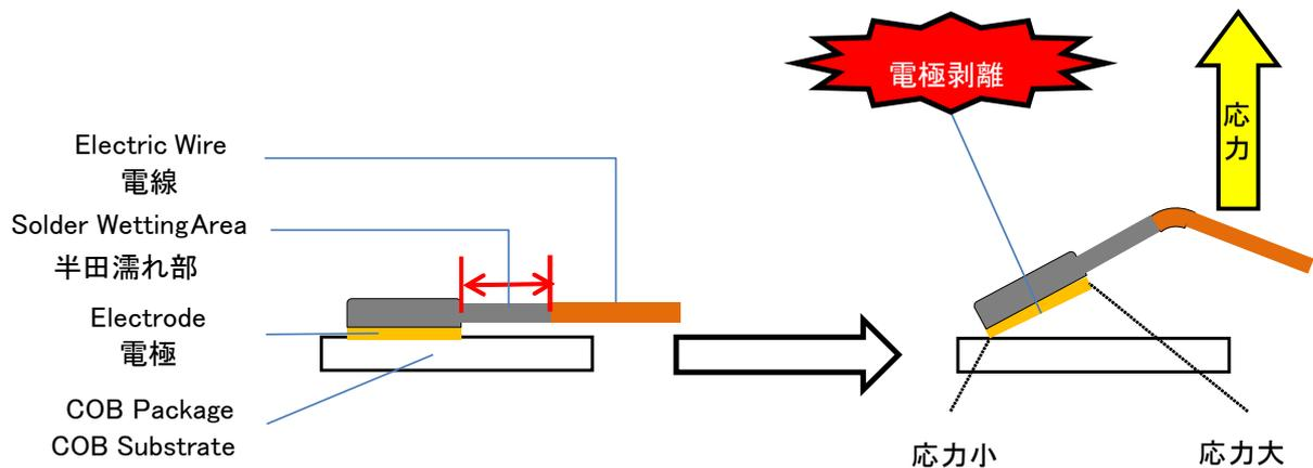
Figure 5. Mechanism of Electrode Detachment by Stress
