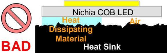
Figure 13. Heat Sinks with Uneven Contact Surfaces and Insufficient Heat Dissipating Material
