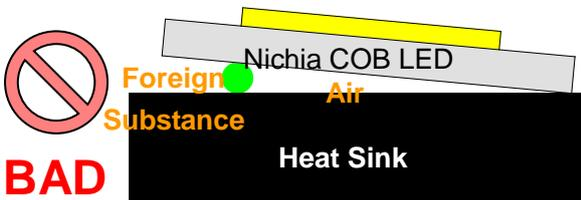
Figure 17. Heat Sinks with Foreign Material on the Contact Surface
