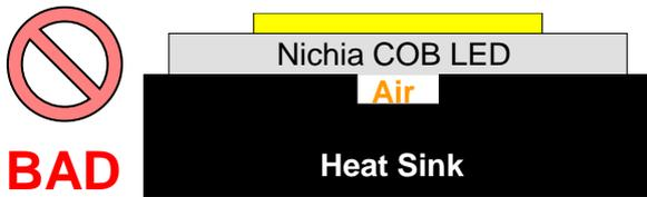
Figure 15. Heat Sinks with Holes/Recesses on the Contact Surface
