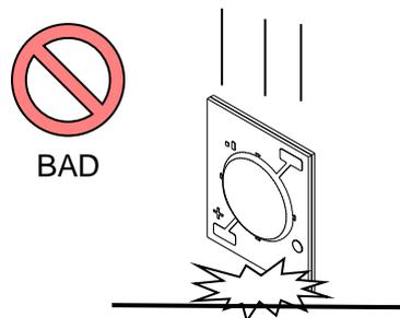
Figure 8. Do not drop the COB LEDs.
