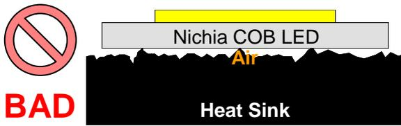
Figure 11. Heat Sinks with Uneven Contact Surfaces
