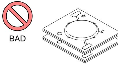
Figure 9. Do not stack the COB LEDs on top of each other.
