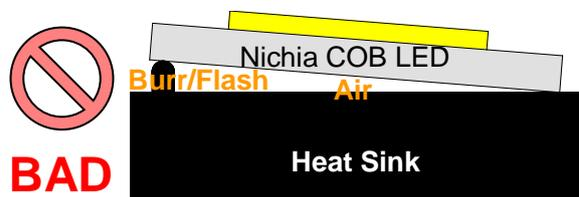
Figure 18. Heat Sinks with Burrs/Flashes on the Contact Surface
