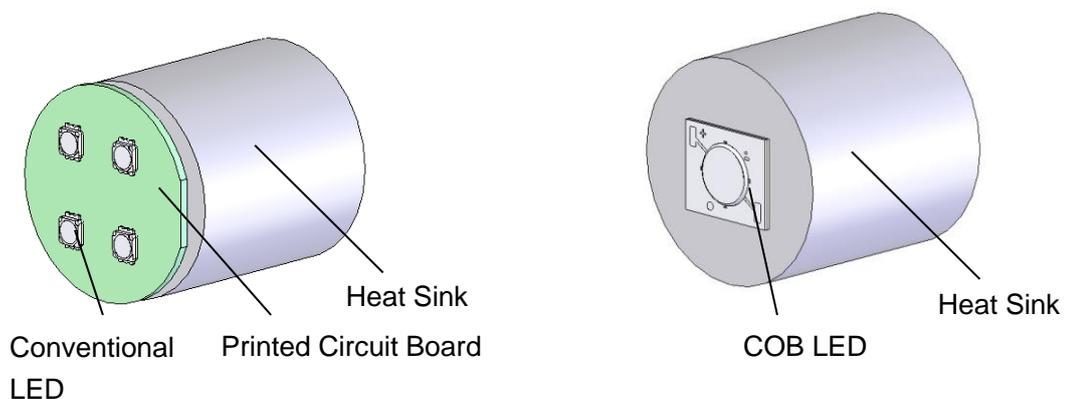
Figure 2. Difference in the Attachment Method to Heat Sink
