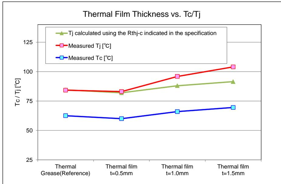
Figure 6. Thermal Film Thickness vs. Tc/Tj
