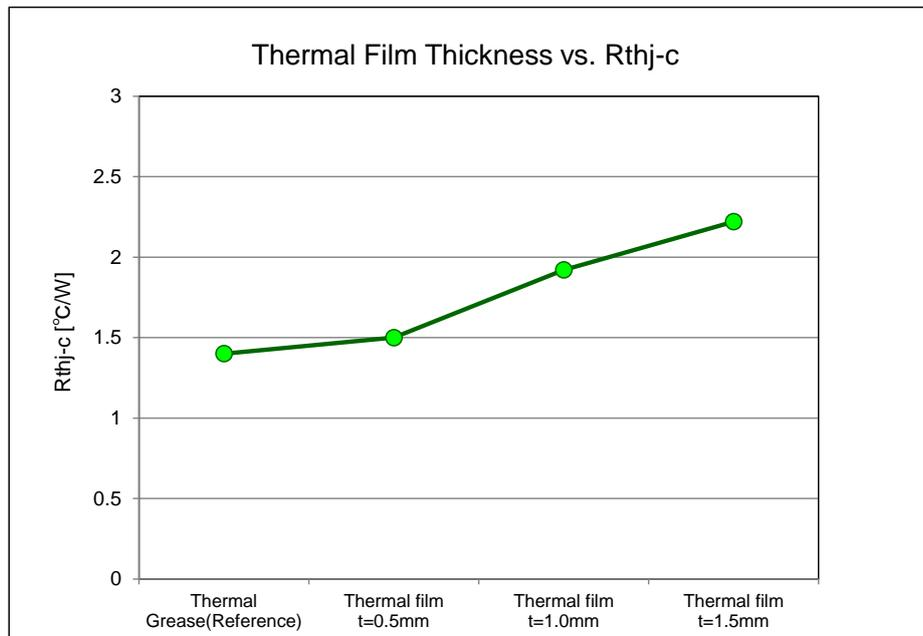
Figure 5. Thermal Film Thickness vs.  $R_{thj-c}$
