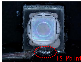
Picture 1 T_s Measuring Point
