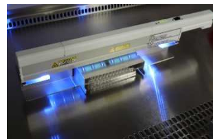
照片 1. Experimental environment (reconstruction) Irradiation conditions: irradiation distance 50 mm, irradiance 1.7 (mW/cm 2 )
