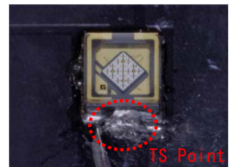
Picture 1 T_s Measuring Point
